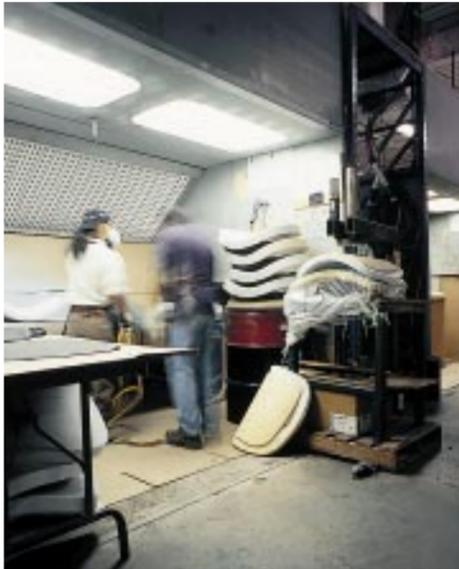
The process used to bond fabric to foam with water-based glue has superior bonding capabilities, which helps to improve the overall quality of Global products. As well, water-based glue dramatically reduces the chemicals used during the manufacturing process.
