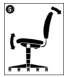
**Tilt**Pivot point located directly above center of chair base (white dot indicates pivot point).
