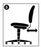
Seat Depth Adjustment Positions chair back relative to seat to reduce pressure on the buttocks and thighs for both taller and shorter users.
